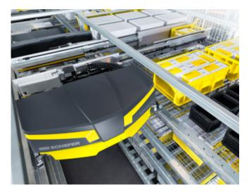
High-density tub and carton storage provided by an AS/RS system allows for sufficient quantity of stored units during peak periods.
