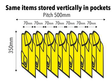
As seen in Figure 7, a T-shirt placed on a traditional sorter takes up a footprint of 600mm x 500mm, despite its comparatively small size. If we take the item and turn it vertically into a hanging sortation system, such as a pocket sorter, one can singulate seven items in the same footprint.
