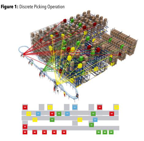
In this graphic, supply tubs carry inventory for specific orders (indicated by like colors) on a conveyor system in front of an automated storage and retrieval system (AS/RS). As the number of orders increases, supply tub traffic coming to a pick station increases, which can create bottlenecks.
