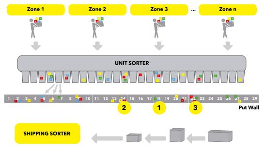
The number of sort/put destinations limit the batch size. This limitation produces a low pick density, unproductive picking, and a large labor force. Inefficiencies compound when large labor forces get too far out of sync and orders cannot be cleared.
