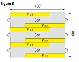
Since most spec buildings today are built at or around 1 million sq. ft., using traditional loop sortation could limit location options and/or reduce speed to market. In the NextGen solution featuring dense automated storage, automated pocket buffering, sequencing, and sortation, the solution can fit into a 1 million sq. ft. spec warehouse by taking advantage of the previously non-productive vertical space inside the warehouse.
